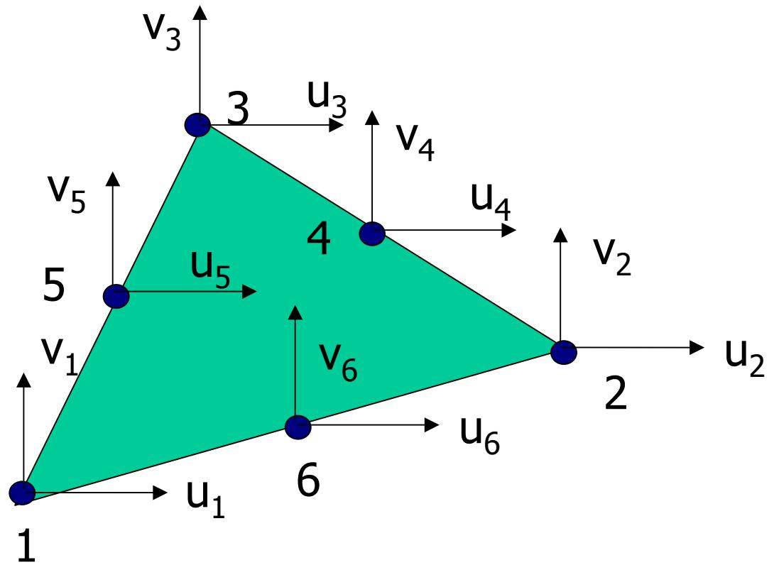
$$\{\delta\} = \begin{pmatrix} u_1 \\ v_1 \\ u_2 \\ v_2 \\ u_3 \\ \vdots \\ v_6 \end{pmatrix}$$
