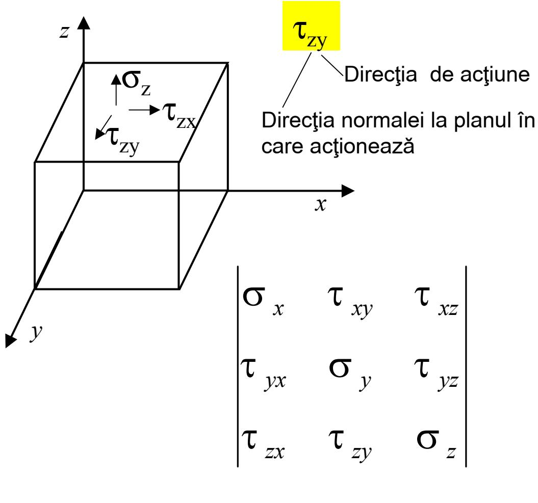
$$\left\{ \begin{array}{l} \sigma_x \\ \sigma_y \\ \sigma_z \\ \tau_{xy} \\ \tau_{xz} \\ \tau_{yz} \end{array} \right\}$$
