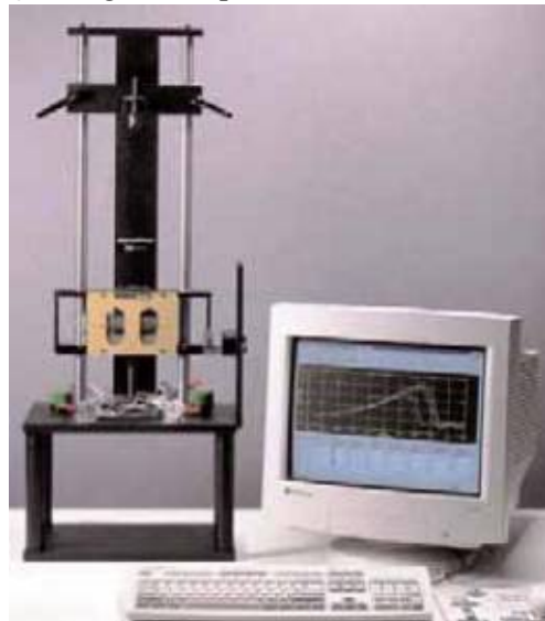
Figura 27 Dynatup MiniTower Instrumented Impact Testing System [9]
